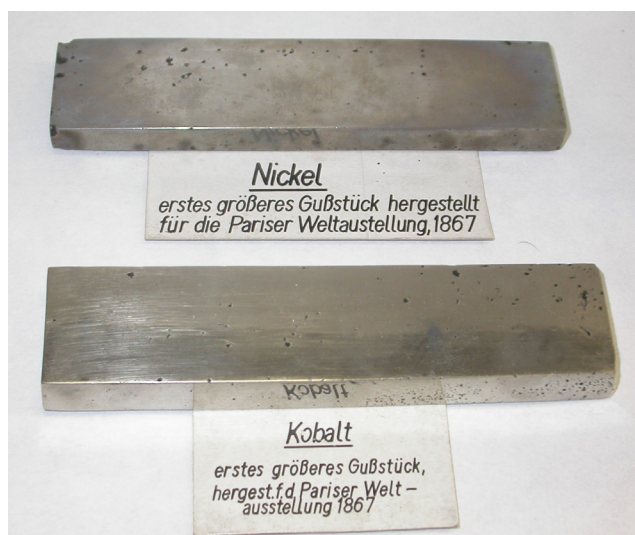
Figure 3. Winkler's castings of nickel and cobalt, presented at the 1867 World's Fair in Paris. Photo courtesy of Prof. Mike Haustein (Nickelhütte Aue GmbH and TU Bergakademie Freiberg).
