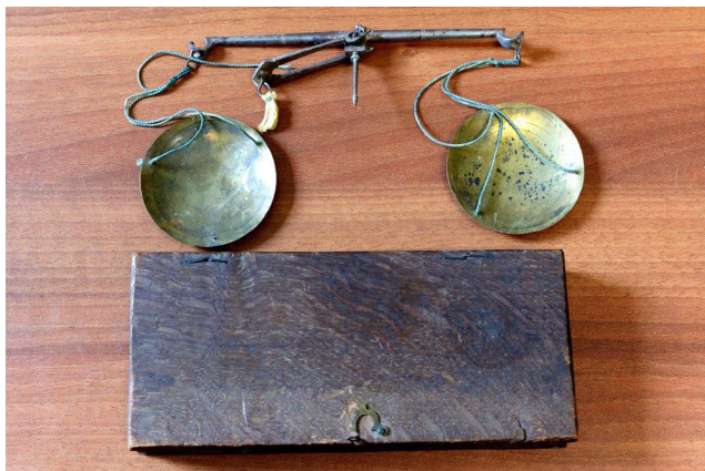
Figure 2. Simple scales for weighing drugs supplied in the Randall & Son medicine chest along with the wooden box which held them along with weights and a business card. Photograph by Richard Johnson.
