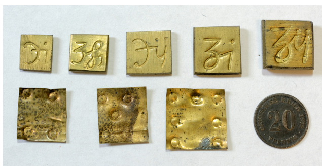
Figure 3. Weights supplied with the scales in Figure 2. Top row (left to right): 1 Scruple, ½ Dram, 2 Scruples, 1 Dram, 2 Drams; Bottom row (left to right): 4 grains, 5 grains, 7 grains; a 20 pfennig 1875 silver coin (1.00 gram) added perhaps 80 years after the set was originally sold. A ½ scruple weight may well be missing. See the text for definitions of these weights. Photograph by Richard Johnson.
