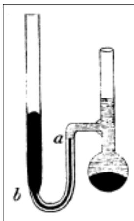
Figure 6. Compact capillary electrometer; Ref. 11, p 555.
