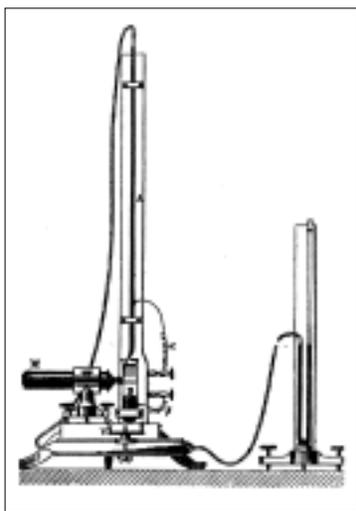
Figure 4. Lippmann capillary electrometer; Ref 5, p 532
