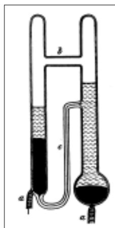
Figure 8. Luther capillary electrometer; Ref. 15, p 426
