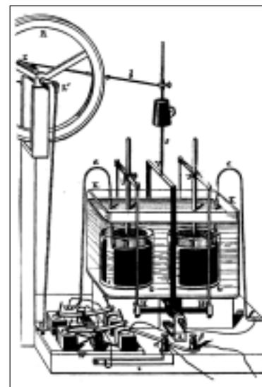
Figure 2. Electrocapillary motor; Ref. 5, p 522.
