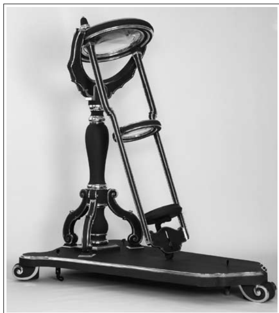
Figure 3. Two-stage burning lens apparatus built by Ehrenfried W. v. Tschirnhaus, in Kieslingwalde around 1690; reproduction (image courtesy of Staatliche Kunstsammlungen Dresden, Mathematisch-Physikalischer Salon, Photographer: Michael Lange, Dresden, reproduced with permission).
