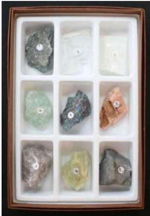
Mohs Hardness Kit: 1=talc, 2=gypsum, 3=calcite, 4=fluorite, 5=apatite, 6=orthoclase, 7=quartz, 8=topaz and 9=corundum. An unknown sample can be “scratched” by the test sample just harder than itself.
